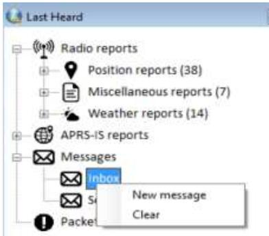
Enter the SSID (Callsign + "hyphen" + "suffix") of the station you want to send a message to. IN this case I will be sending to my mobile rig from my base station: AG7GK-9
